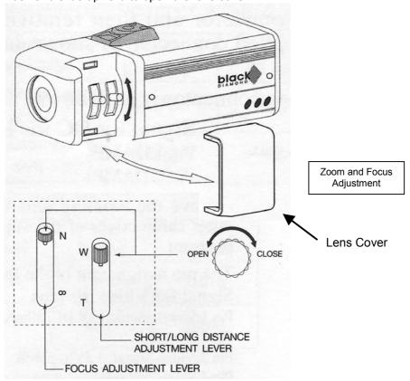
To adjust focus and the viewing angle (Zoom) you have to loosen the adjustment lever by turning left, afterwards you can slide the adjustment lever up and down.
